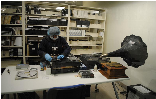
Fig. a) Magnetic tape cleaning
